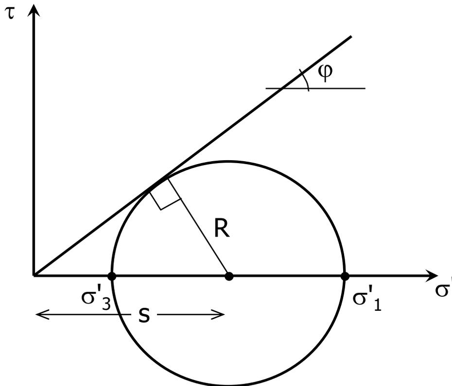
$$R = \frac{\sigma'_1 - \sigma'_3}{2} = s \cdot \text{sen} \varphi' = \frac{\sigma'_1 + \sigma'_3}{2} \cdot \text{sen} \varphi'$$
