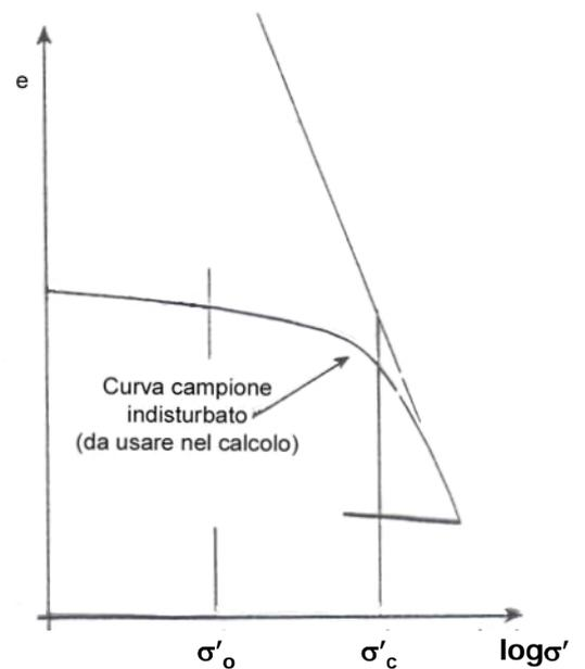
$$\Delta e = C_c \cdot \log \frac{\sigma'_{v0} + \Delta \sigma'_z}{\sigma'_{v0}}$$
