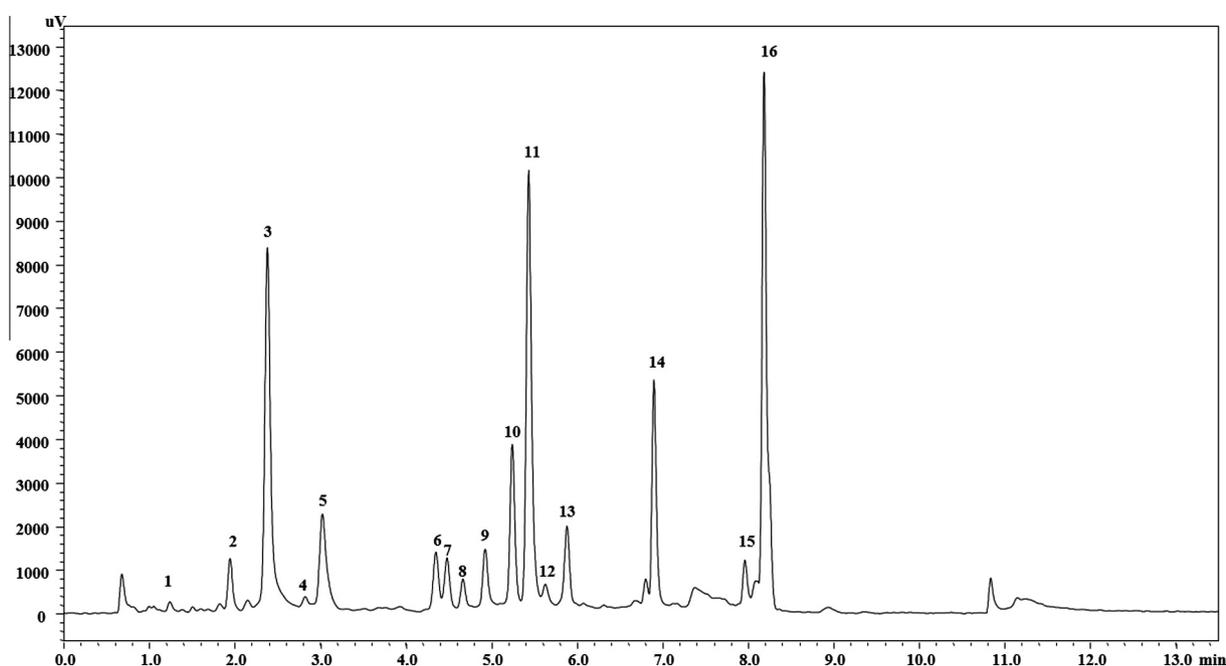
Fig. 1. UHPLC–PDA chromatogram of green lettuce polyphenolic extract, column: Kinetex C18 150 × 4.6 mm, 2.6 µm, flow: 2.2 mL/min, inj.vol 2 µL, column oven 48 °C.
