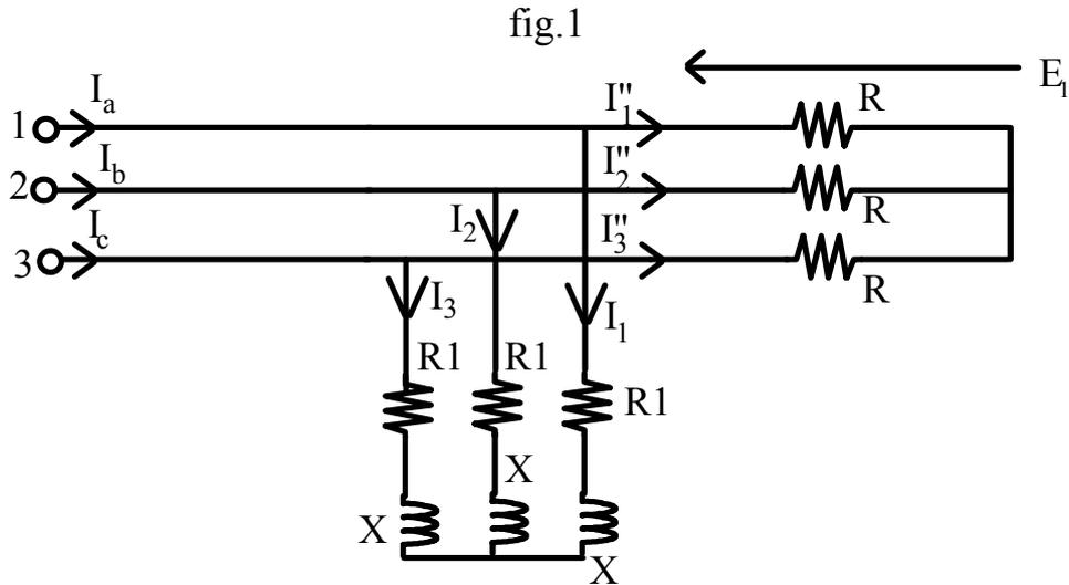
$v_{12}(t) = \sqrt{2} \cdot 380 \cdot \sin(314 t)$ ;  $R_1 = X = R = 10 \Omega$ ;
