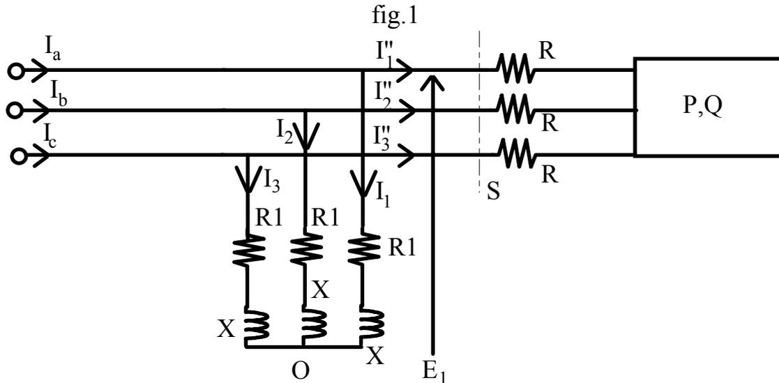
$i''_1(t) = \sqrt{2} \cdot 5 \cdot \sin(314 t)$ ;  $R_1 = X = R = 10 \Omega$ ;  $P = 1 \text{ kW}$ ;  $Q = 1 \text{ kVAr}$ ;
