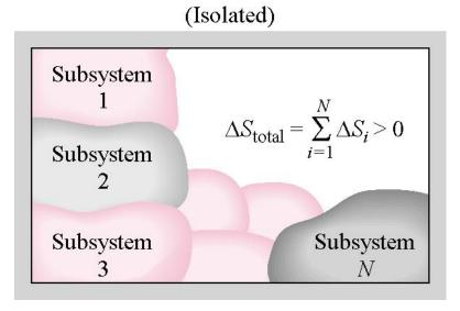
Applying the definition of entropy to the isolated system
