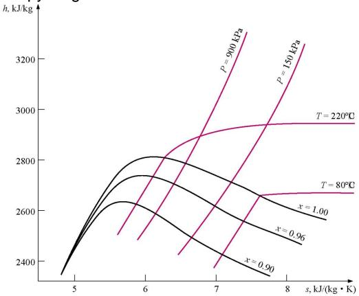
Shown above are the temperature-entropy and enthalpy-entropy diagrams for water. The *h*-s diagram, called the Mollier diagram, is a useful aid in solving steam power plant problems where heat transfer and work may be expressed as enthalpy changes for steady-flow constant pressure and isentropic processes, respectively.
