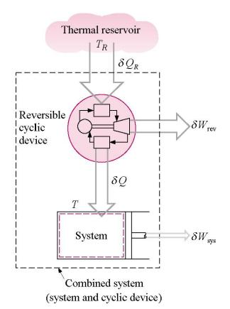
We apply the first law on an incremental basis to the combined system composed of the heat engine and the system.
