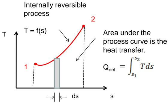
In the above figure, the heat transfer in an internally reversible process is shown as the area under the process curve plotted on the T-S diagram.
