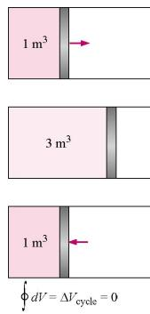
When the piston returns to its initial position at the end of a cycle, the volume of the gas also returns to its initial value. Thus the net change in volume during a cycle is zero. This is also expressed as
